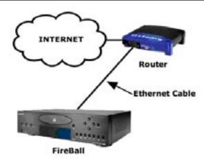
CAT5 cabling should not exceed 100 meters. The following drawing depicts the typical wiring scheme for CAT5.
